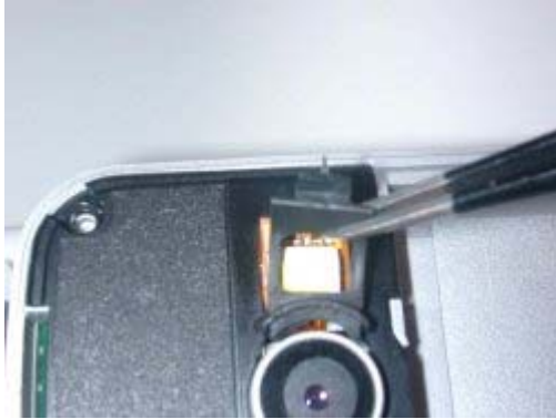
Take out the camera gasket with tweezers
