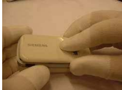
Shift the cover (be careful with plastic pin )
