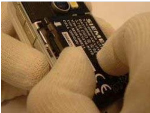
Take out the battery pack by releasing the 2 fingers from their catches and lifting the battery Upward from the strip.
