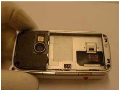
Unscrew the four screws of the mounting frame
