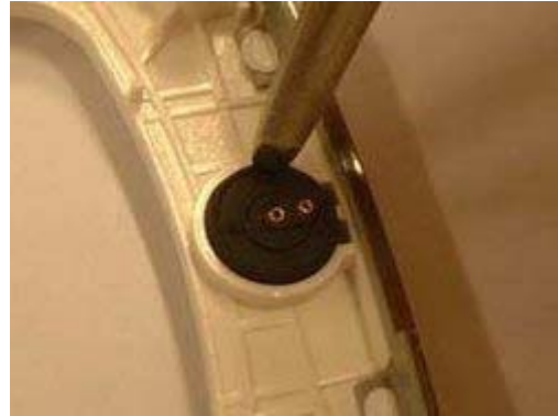
Place the microphone with tweezers
