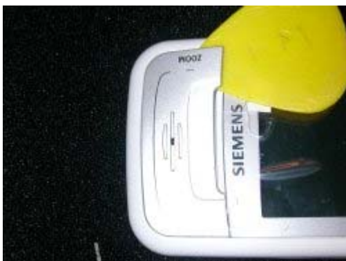
Remove the zoom key by lifting it upward
