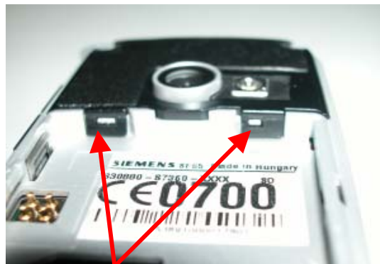
Release the antenna with connectors by pushing the antenna fixing fingers
