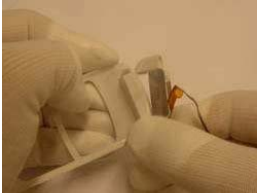
Carefully pull out the flex (pay attention not to damage it )
