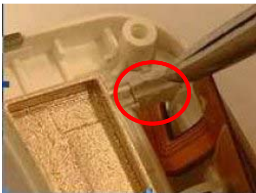
Place the white cap next to the screw bordering
