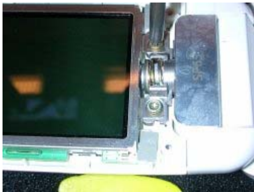
Unscrew the two screws of the LCD module
