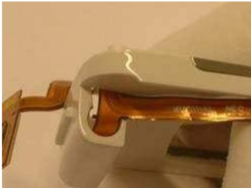
If necessary push with a plastic tool to release the flex cable
