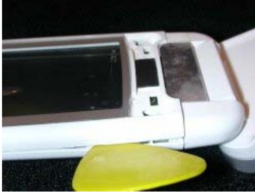
Separate the flip front case from the flip rearcase
