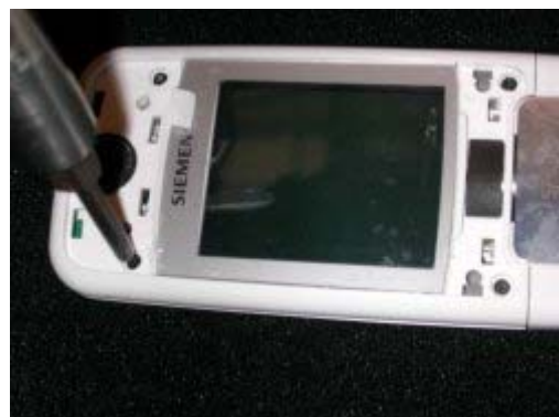
Unscrew the four screws of the flip front case
