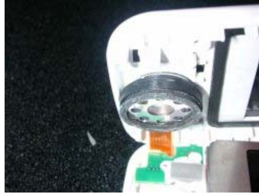
Open the covers (be careful, earphone is stuck on the top and bottom)
