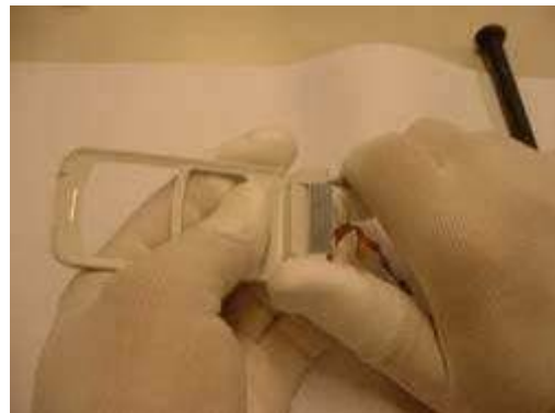
Hold spring compressed in the hinge. When the hinge is released, remove the hinge body
